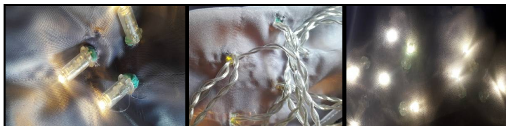
Fig (6) LED fixed in the front of satin lining Fig (7) LED wires at the back of satin lining Fig (8) chiffon fabric on LEDs
