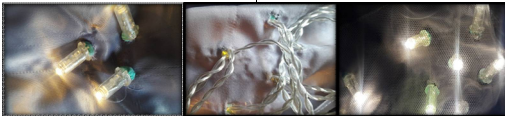
Fig (1) LED fixed In the front of satin lining
